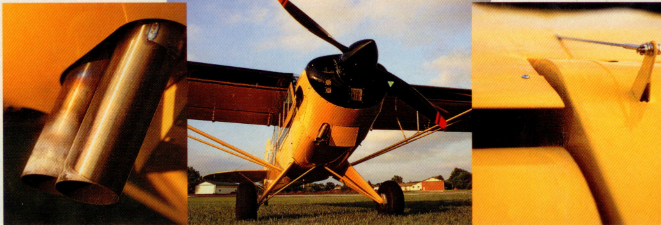
A more powerful engine with dual exhaust, a composite prop, and a redesigned wing with extended flaps and dynamically balanced ailerons take the airplane to a new level in the bush. Performance has improved all the way around.
